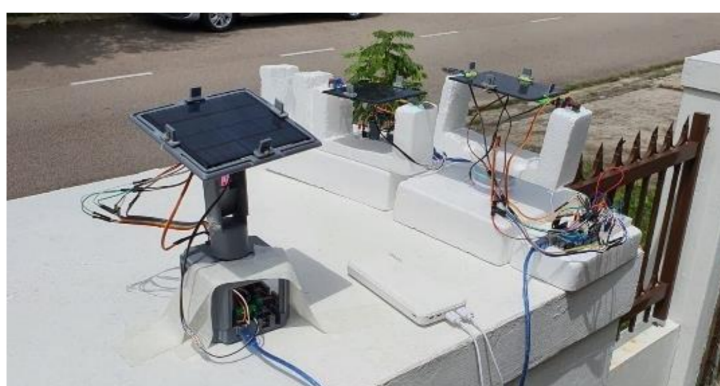
Figure 5: Experiment of Collecting Instantaneous Power at Each Period
