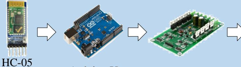
Arduino Uno **Motor Driver** Bluetooth Module
